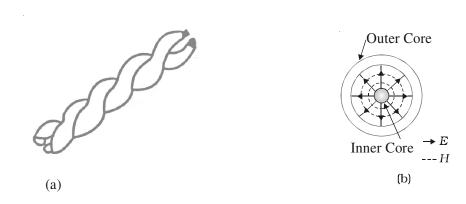
Figure 33.1: (a) A twisted pair (b) A coaxial cable
